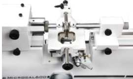
Calibration of Effective Diameter of an External Thread
