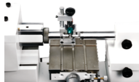
Calibration of Plain Plug Gauge
