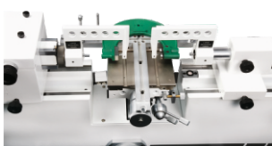
Calibration of Snap Gauge
