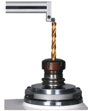
Checking of a Height
