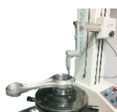
For measuring the roundness & parallelism of the small and large ends.
